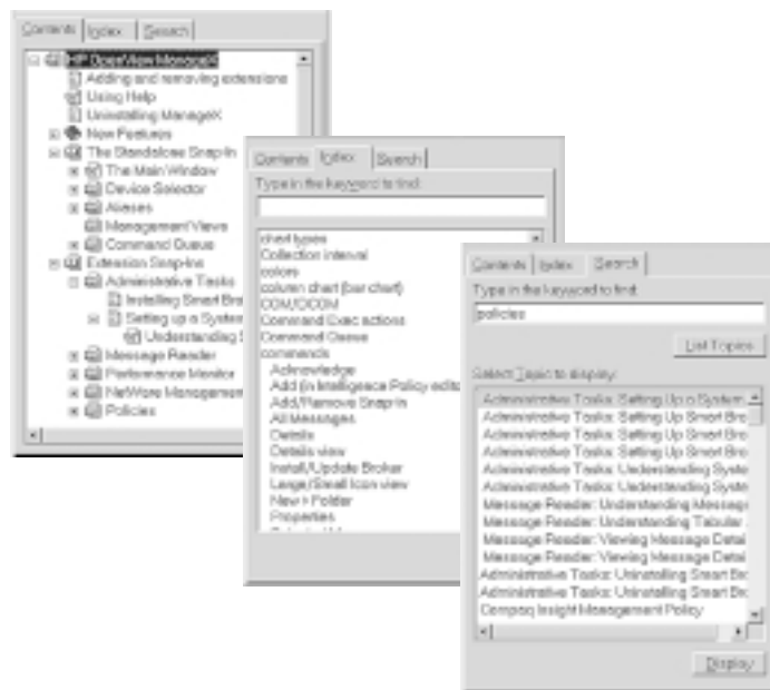
Figure 2.2 Basic HTML Help Navigation Pane. Compiled HTML Help uses a “tripane” format with the left pane devoted to navigation tabs. The three standard tabs are the Contents, Index, and Search tabs. A Favorites tab is also available for storing users’ most frequently referenced pages.
